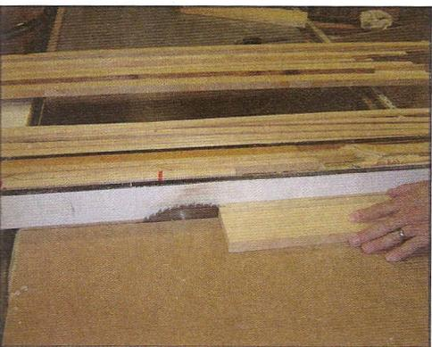
*Feeding thin strips through a saw can be dicey. So each cut stops 6 inches short of the end of the board. Then the board is reversed and cut from the other end while holding it tight to the fence. Same thing is done when the wide pieces are laid flat and ripped to 1/4 inch square. This saves fingers.*
