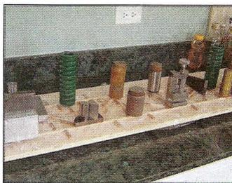
*Gussets are glued to the top side with a light weight to hold each in place as the glue dries. Gussets are not nailed or stapled, and clamping pressure is fairly light.*
