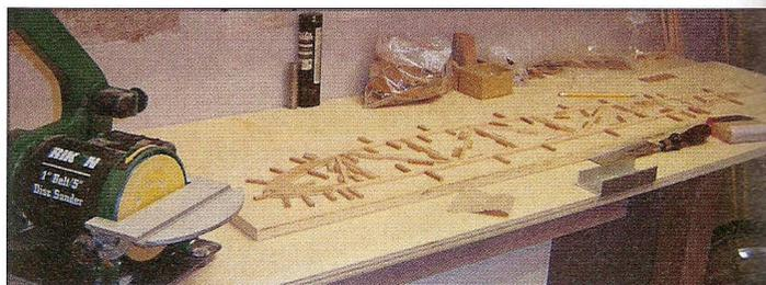
*Rick said he cuts each capstrip and finishes it to dimension with a small disc sander. He explained, "After all pieces are fit, I then remove them all and place Glad Cling Wrap over the rib jig, then replace all of the capstrips, gluing each as they are put into the jig. Cling Wrap allows for easy removal of the rib after the glue sets."*
