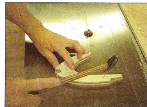
*Make an exact hardwood, or birch ply, template of the nose rib and tack it to the rough-cut rib blanks.*
