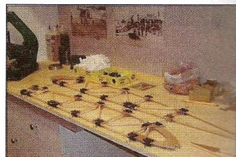
*With the back side sanded, the other gussets are glued in place. Paper clips make a great clamp for this application. The excess gusset material is routed off, and the rib is finished.*
