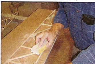
*A sanding block is used on the reverse side to level the surface and remove any excess glue.*
