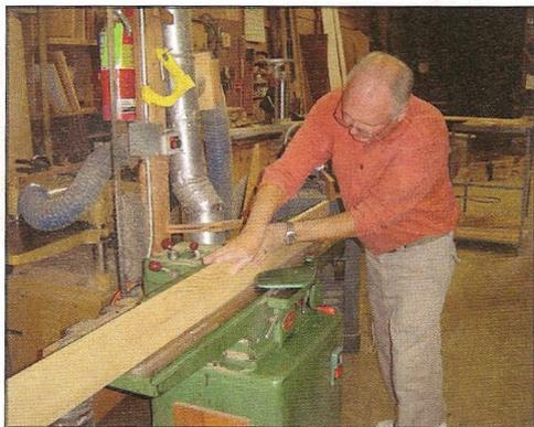
*True one edge of a straight grain spruce or Douglas fir plank on a jointer. A hand plane will also do the trick. Don't chintz on the lumber quality. Any serious grain run-out or wide grain will come back to haunt you later.*
