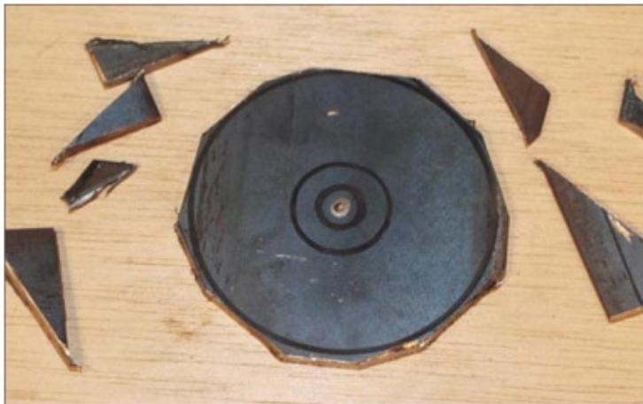
After a few minutes of cutting with the zip disc, the rough cut part is liberated from the flat. Notice how none of the cuts are inside the marked line.
