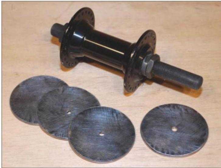
Once all four discs are rounded and checked to be the same, the edges and mill scale is cleaned up using a flap disc, which is a grinder disc with sandpaper strips attached to it. The discs are now smooth, clean, and perfectly round. The punched centers have also been drilled using a 1/8 drill bit.
