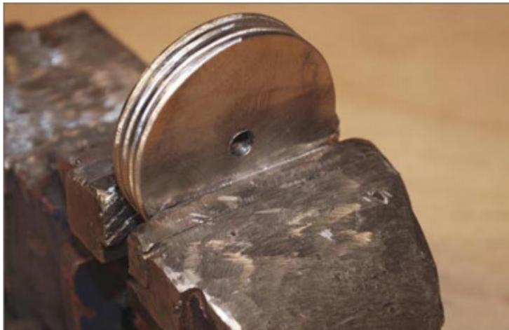
Like I said before, I love to work with minimal tools, and do not own a lathe, chop saw, or even a drill press, so I do my drilling in a vice using a hand held drill. To ensure that all four discs have the hole
