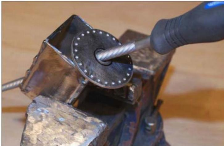
After drilling, the four discs ready to have the centers hand filed to 3/4 inch diameters. The discs are very accurate considering they were carved from a \$3 piece of hardware store flat bar using only a hand held angle grinder!
