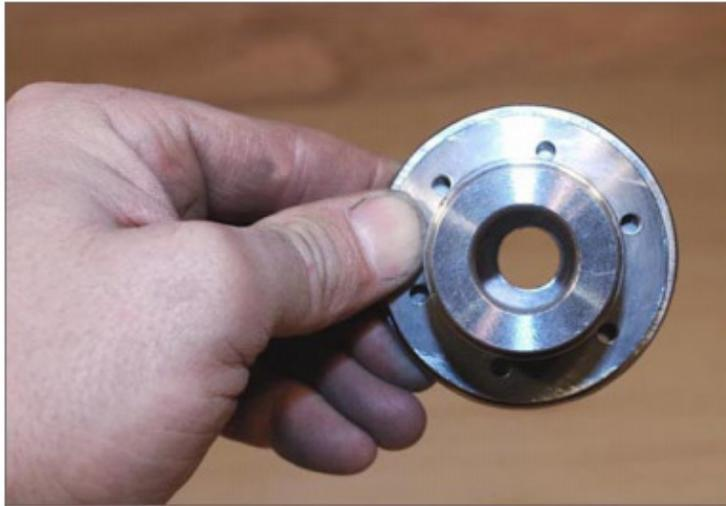
Using a hand drill limits your drill bit size to about 1/2 inch diameter, so the 3/4 inch hole needed for each disc will have to be done using a hand file. This actually works out well since the holes are not perfectly centered as can be seen in the comparison with the hub adapter in the photo. Using the paper template and a round file, the 3/4 holes will be hand filed. This procedure only takes a few minutes per disc but is extremely accurate.
