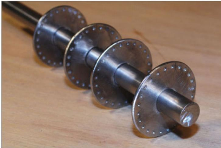
An hour later, all 4 discs fit snugly on the 3/4 axle as shown in the photo. The hand filed holes are actually tighter than the last set I had made at the machine shop. Nothing beats old fashioned hard work!
