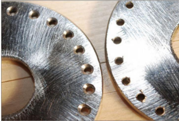
This photo shows the completed beveling of the spoke holes (left side) as compared to the freshly drilled holes (right side). Notice the sharp edges and burs left over from drilling on the unbeveled flange.
