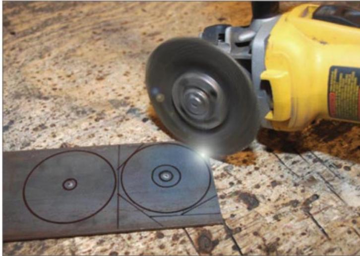
As shown, the discs being cut from the flat bar using a few straight cuts around the circumference with a zip disc. 8 or more cuts are made just outside the marker line so that final grinding does not take much time.
