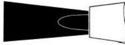
Fig 4-1. The neutral flame, which results from burning a mixture containing approximately equal volumes of oxygen and acetylene. The well-defined core of the flame (extremely bright pale blue) is known as the "inner cone".
