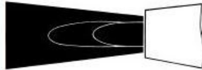
Fig. 4-2. The excess acetylene flame, which has a whitish feather around and beyond the inner cone.
