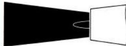
Fig. 4-3. The oxidizing flame, which results from an excess of oxygen in the gas mixture, has a shorter, more sharply-pointed inner cone than the neutral flame.
