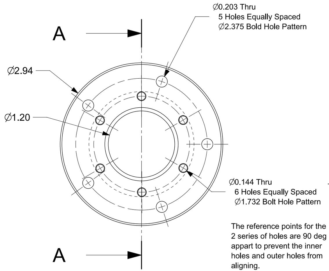
The reference points for the 2 series of holes are 90 deg apart to prevent the inner holes and outer holes from aligning.
