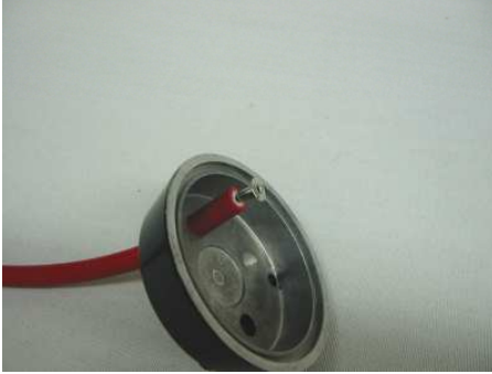
7. Install insert/rivet on center conductor.
