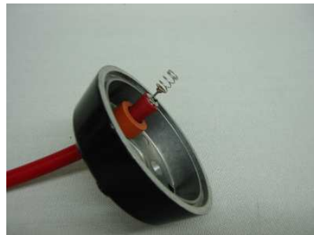
13. Insert carefully not to bend the contact spring pin.
