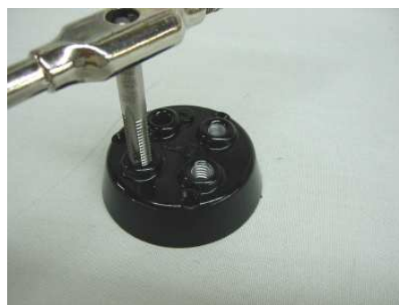
4. Tap hole to 3/8" x 16 coarse thread pitch. Chamfer holes each side. De-burr threads lightly.
