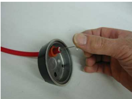
12. Use a tee-pin to create a provision space/hole next to the center conductor and the insert's inside wall for the contact spring pin to be inserted into.
