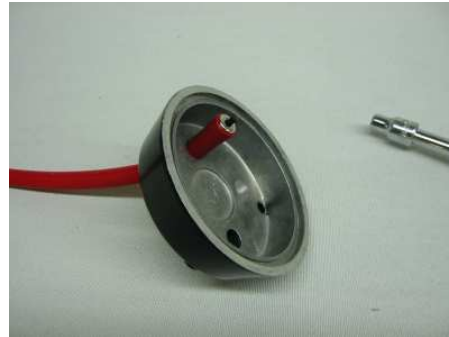
10. Seat completely and cut off center conductor flush.
