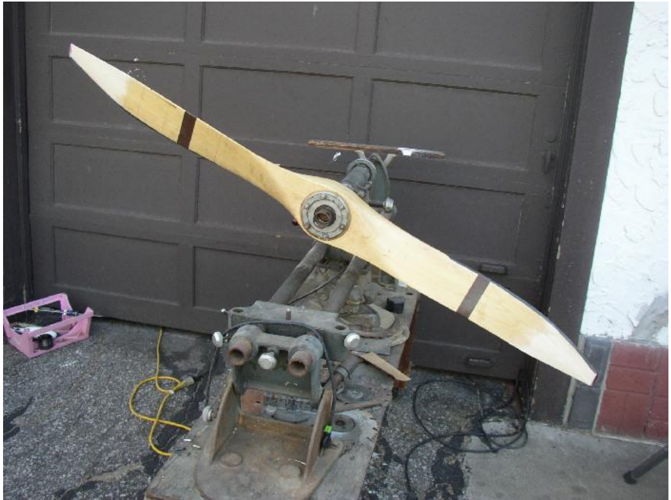
Balance and refinish the tips. I do it on an ancient Shopsmith, with propeller installed on the hub.
