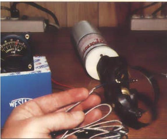
Another type of probe is heated by the torch and shows the temperature on the EGT gauge.
