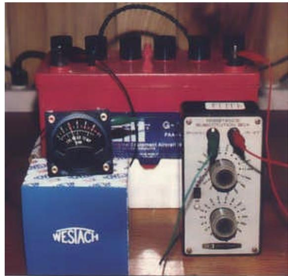
A 12-volt battery and a resistance substitution box makes testing CHT and EGT meters easy. Don't use too little resistance!
