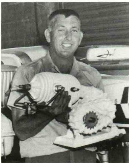
Turbonique, Incorporated, an Orlando, Fla. firm, has just announced the availability of six new turbine engines. These engines cover a guaranteed power range of from 45 to 360 shaft horsepower. The engines are exceptionally lightweight. The smallest unit weighs only 35 lbs. and the largest 55 lbs. This fantastic hp/weight ratio is unprecedented in the commercial, marine, or industrial engine field. Prices are said to be lower than most marine engines and competitive with automobile engines.
