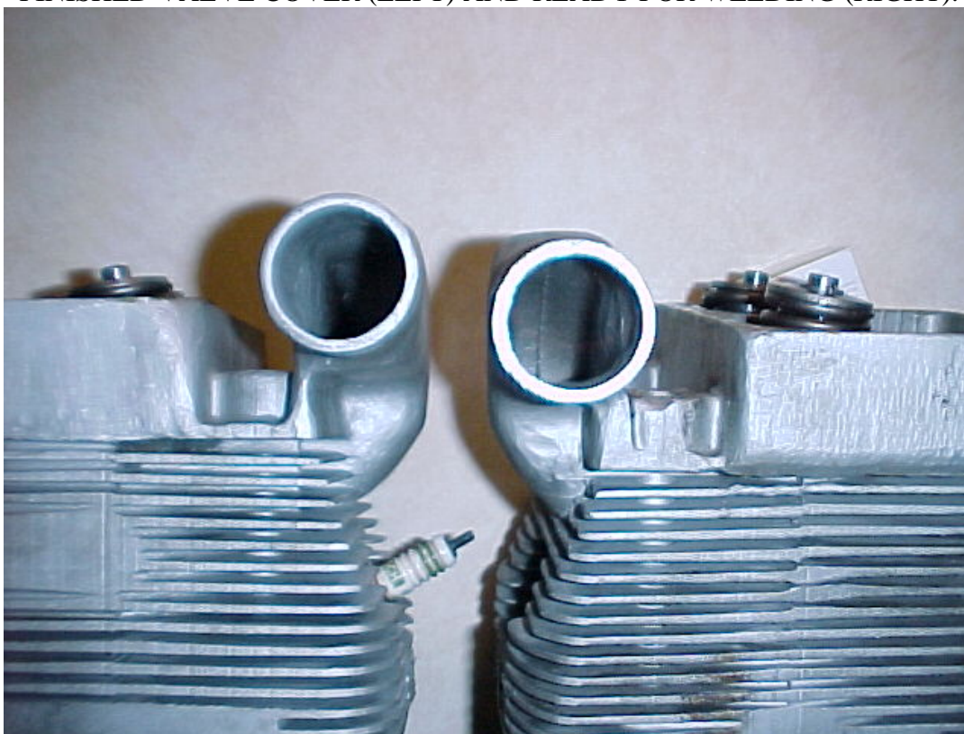
BLEND OUT INSIDE OF INTAKE PORTS.
