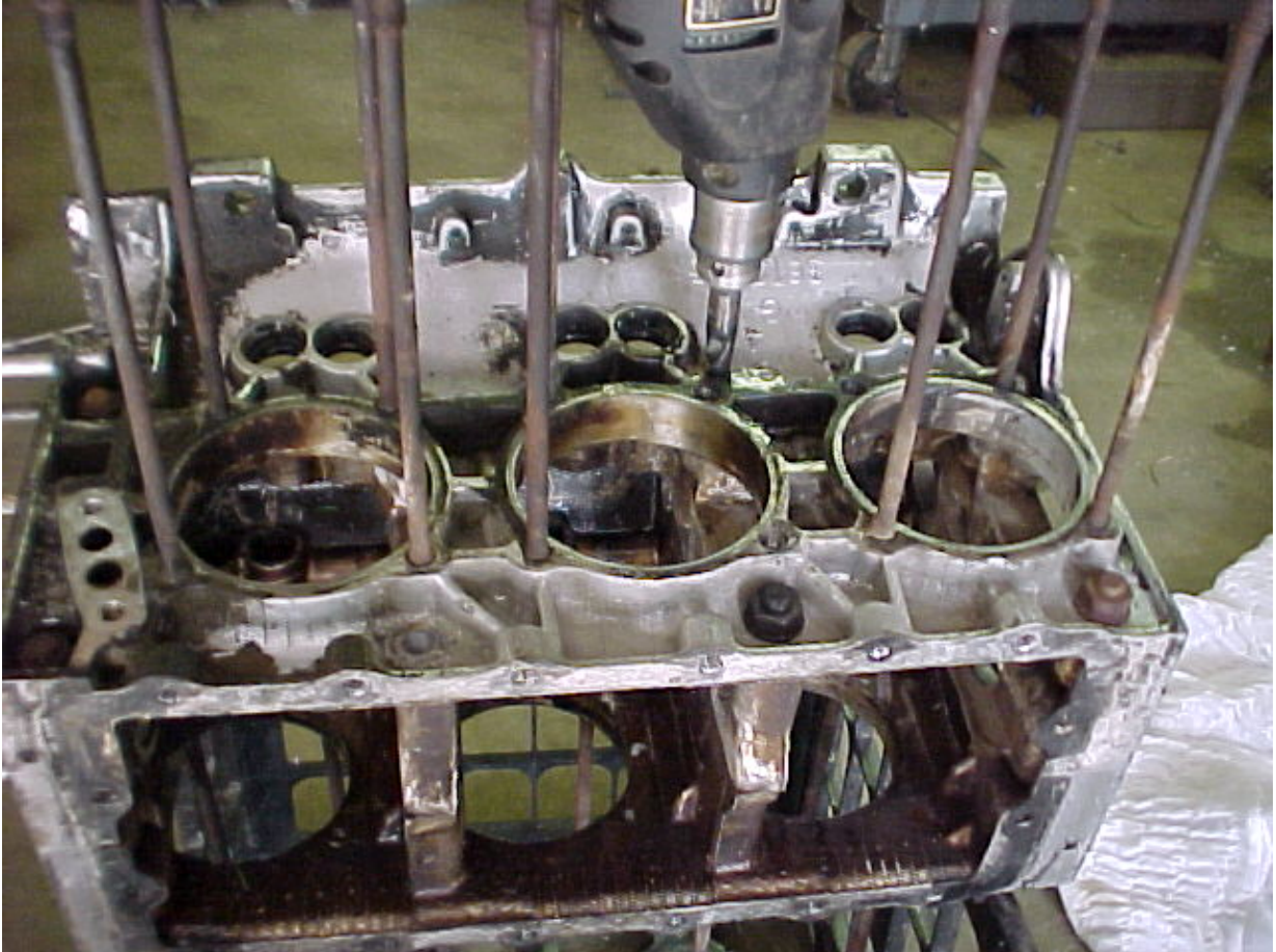
CASE HALVES BOLTED TOGETHER AND DRILLING AT LEAST ½ INCH PAST ENGINE CENTER LINE INTO RIGHT SIDE OF CASE.
