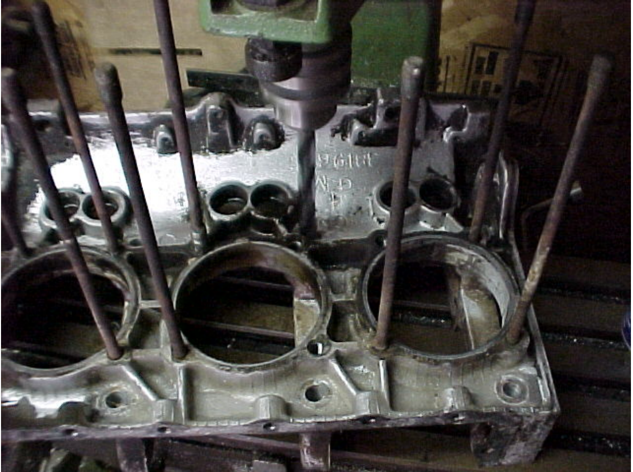
LEFT SIDE CASE BOLT HOLE BEING DRILLED ON A DRILL PRESS WITH A ½ INCH DRILL BIT.
