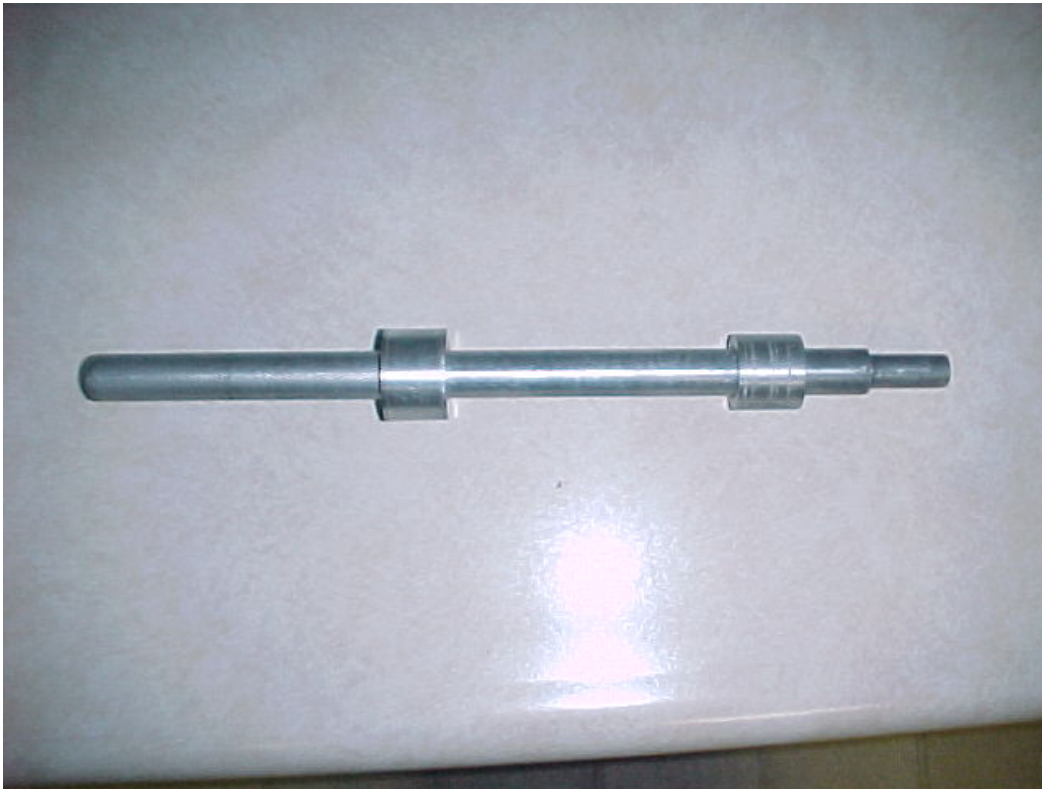
OIL PUMP ALIGNMENT TOOL.
