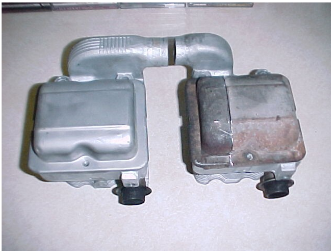
FINISHED VALVE COVER (LEFT) AND READY FOR WELDING (RIGHT).
