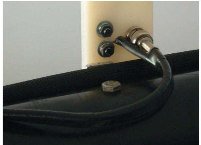
Figure 17 – Spiral wrapped Pawsey Stub.
