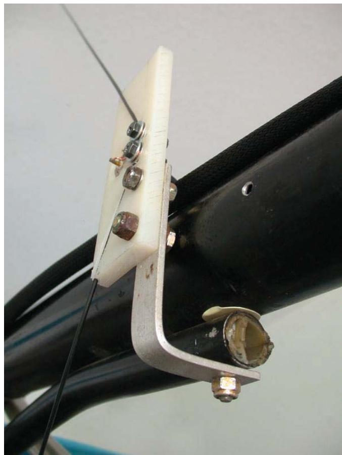
Figure 14 – Antenna mounting example using an L-bracket. Anything similar will work as well.
