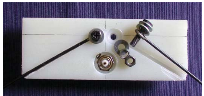
Figure 8 – Mounting the antenna elements and BNC connector.
