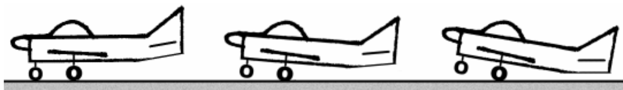
Figure Seven – Elevator angle to airflow during nose pitch down.
